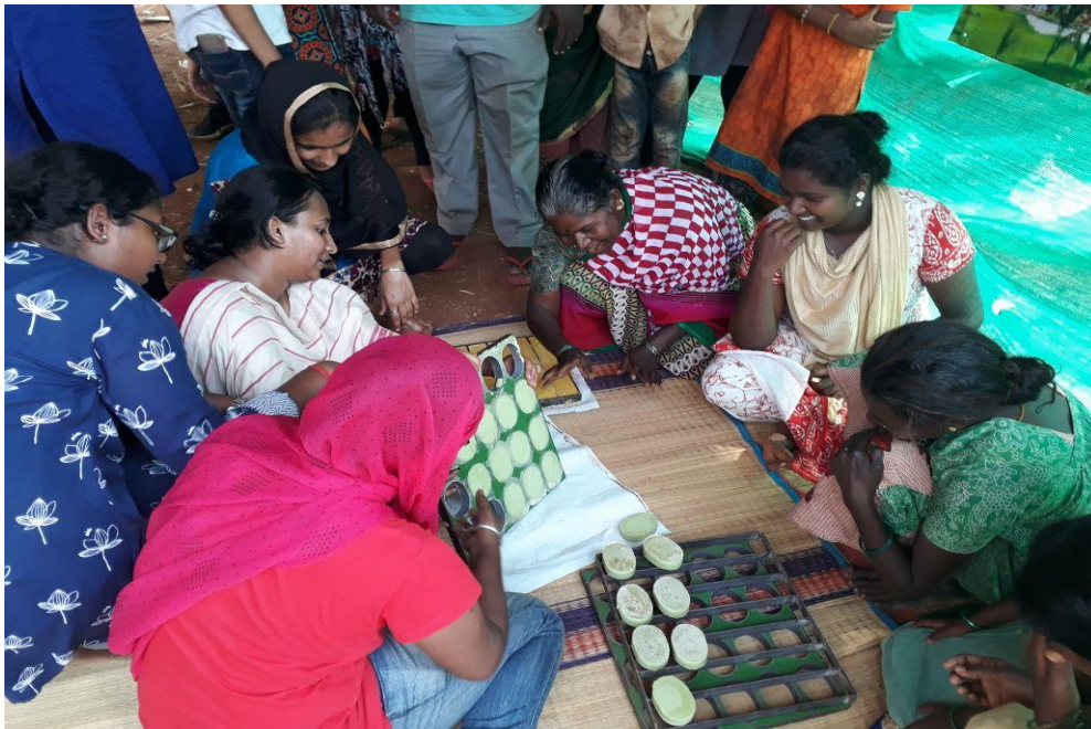
SOAP BEING REMOVED AFTER CURING ON THE FOLLOWING DAY (26.03.2018)
