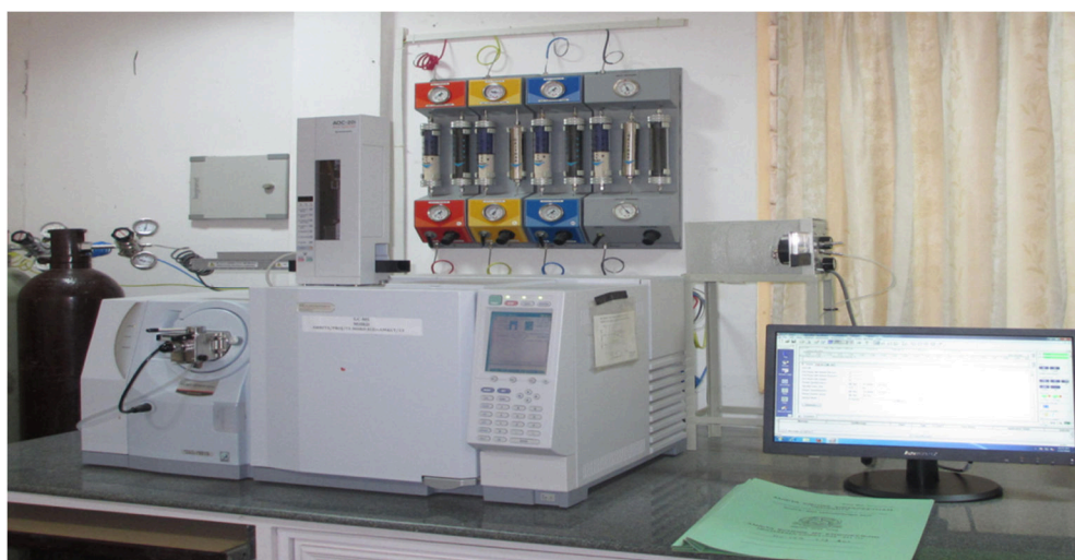
Gas chromatography mass spectrometer (Schimadzu, Japan -QP2010)
