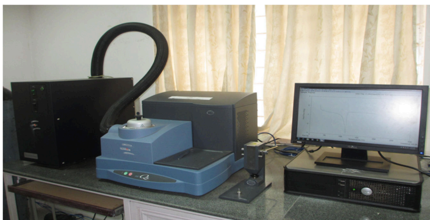
Differential scanning calorimeter (TA Instruments, USA-DSC Q20)
