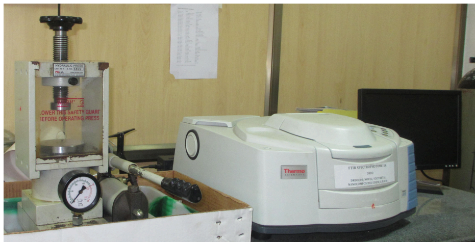
Fourier Transform Infrared spectrometer (Thermofisher, USA- Nicolet iS10)
