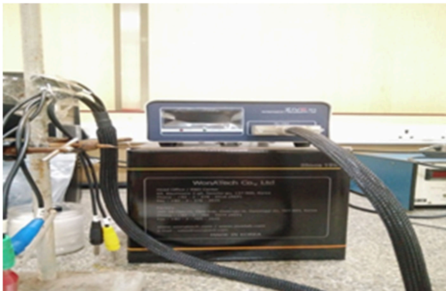
Electrochemical Potentiostat/Galvanostat (Zive SP)
