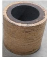
Copper FGM for bearings and bushes
