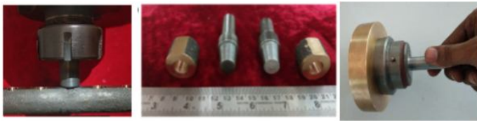
Solid state -friction welding of cast iron and phosphor bronze
